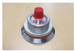
Airtech's Vac Valve 402A is a reusable, high temperature vacuum connector that allows a quick and reliable way to connect vacuum hoses to vacuum bags. The four piece design of this high temperature vacuum connector allows for a tighter connection with an increase in autoclave pressure. When assembled, controlled force is applied to the pressure plate and a solid and reliable air-tight seal is formed.
